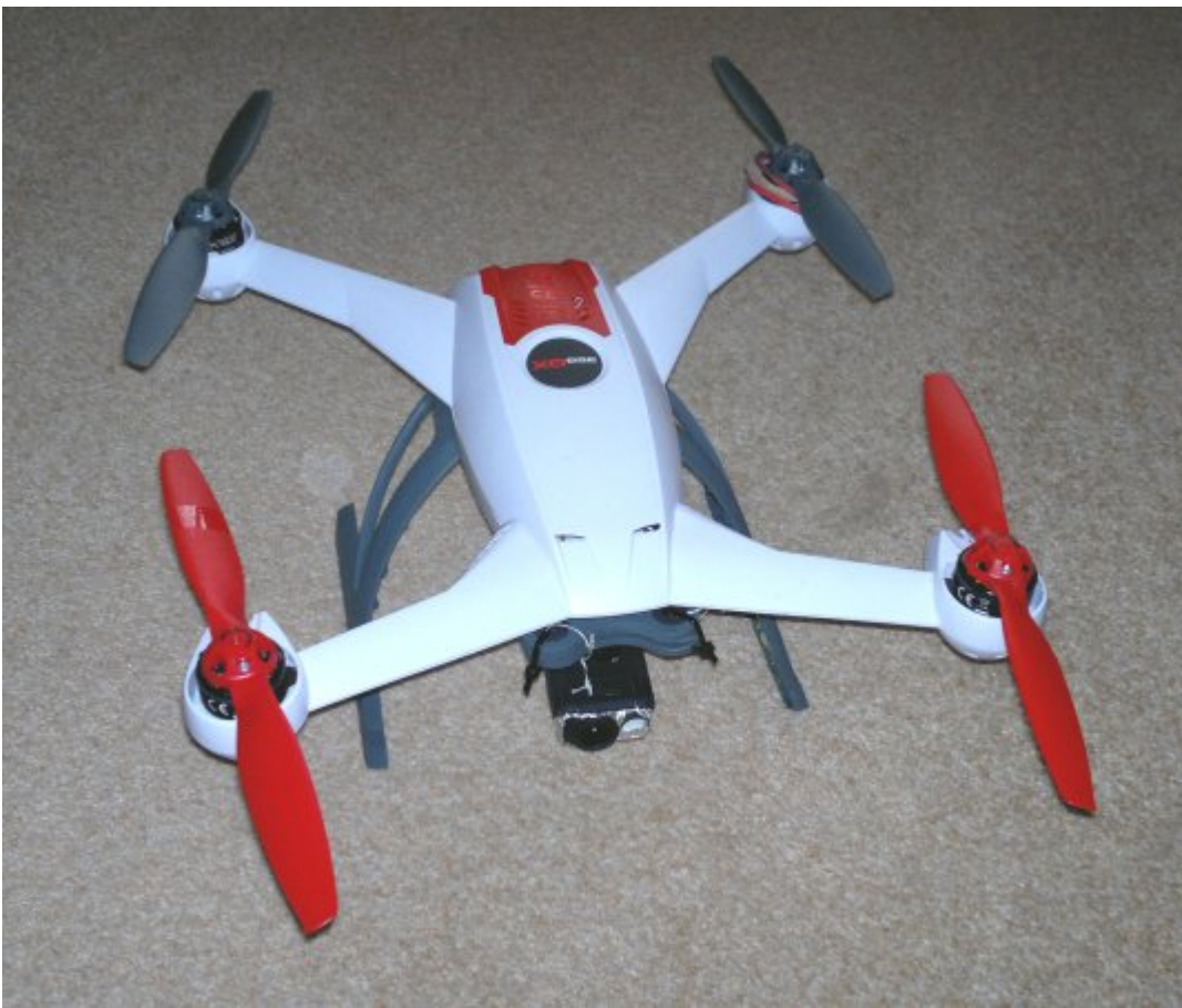
Above - Camera and 5.8GHz downlink Left - Blade 350QX Quadcopter
