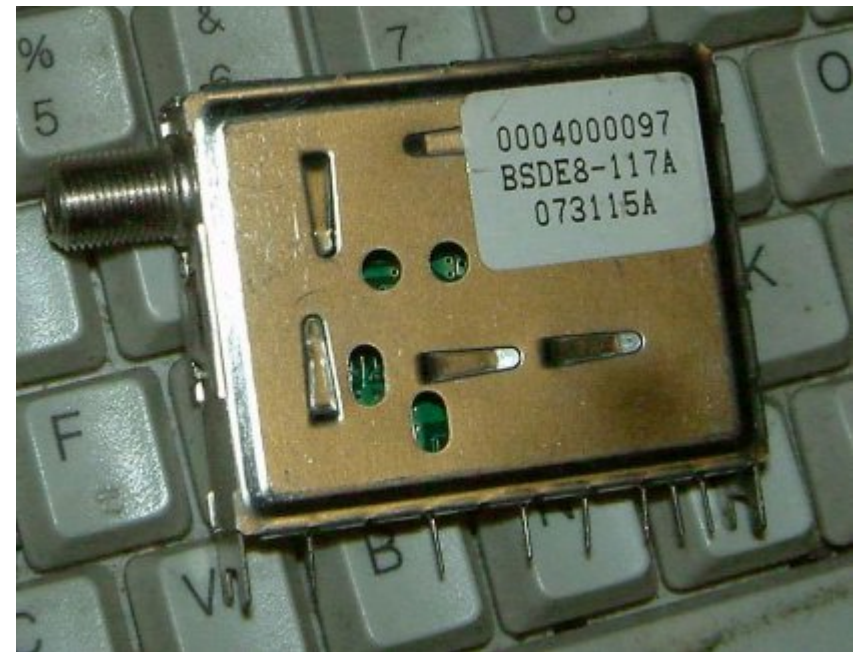
Fig 12 The receiver module, 950-2150 MHz to 480 MHz IF
