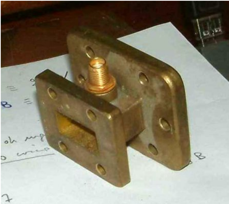
Fig.25 The power monitor with Sma outlet for AGC
