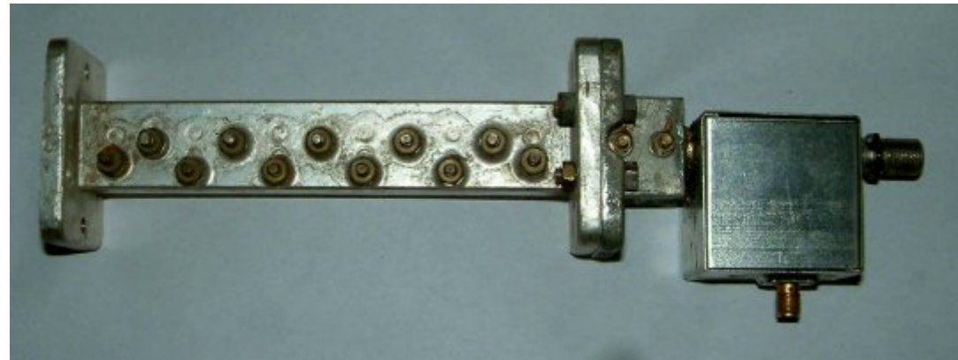
Figure 21 Surplus Mixer and 10 GHz filter
