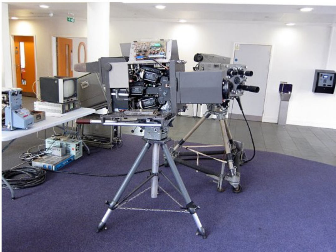
Marconi MkVII with the Marconi MKIII in the background famous for its beer pump focus handle, which was very popular with TV camera men, perhaps for the wrong reason it was dropped and only used on the MKIII
