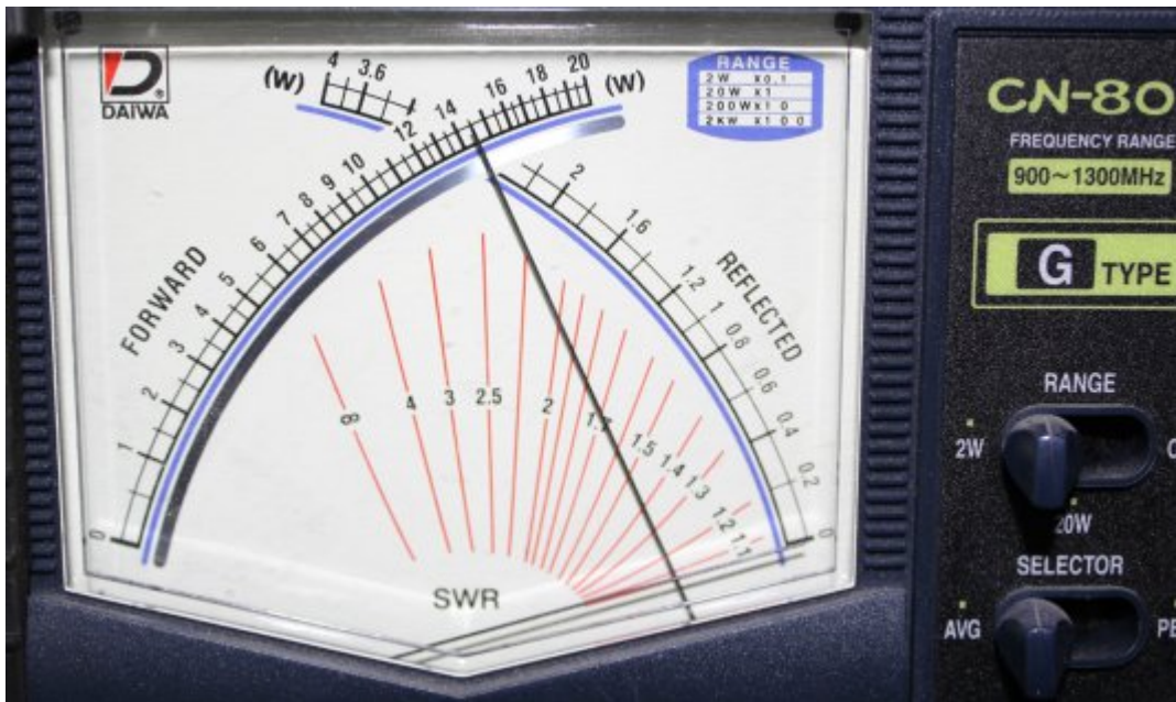
Just 1.45 Watts into VK3RTV2 for a steady picture, QRP ATV, with low VSWR, at work QTH
