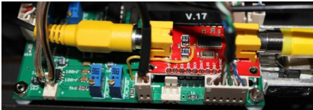
On Screen Display Board, An EMDRC project by Ralph VK3LL and Damian VK3KQ
