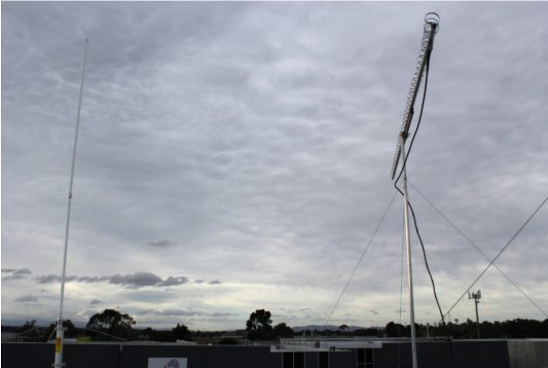
ATV 23cm TX Loop beam pointing to VK3RTV, near Mount Dandenong, in the distance
