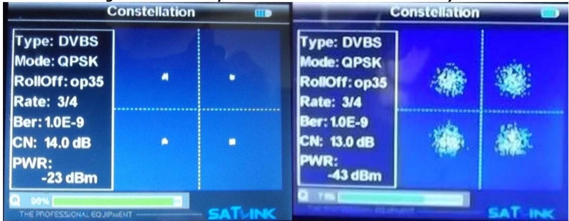
Fig 2 – On the left is the clean QPSK Constellation from new second board layout; on the right is the noisy QPSK Constellation from original board etch layout
