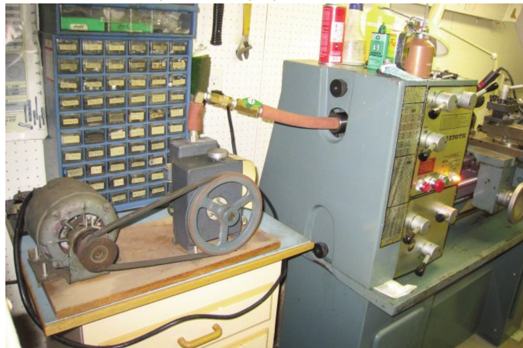
Fig-1 Vacuum pump connected to the lathe
