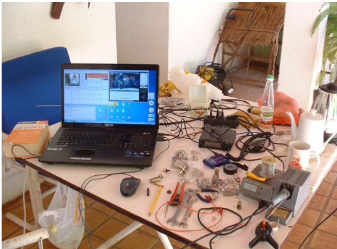
Patio table in Caacupe, Paraguay, RX: TM732E, laptop computer with MMSSTV V1.13A for SSTV reception from ISS on 145,800 MHz FM
