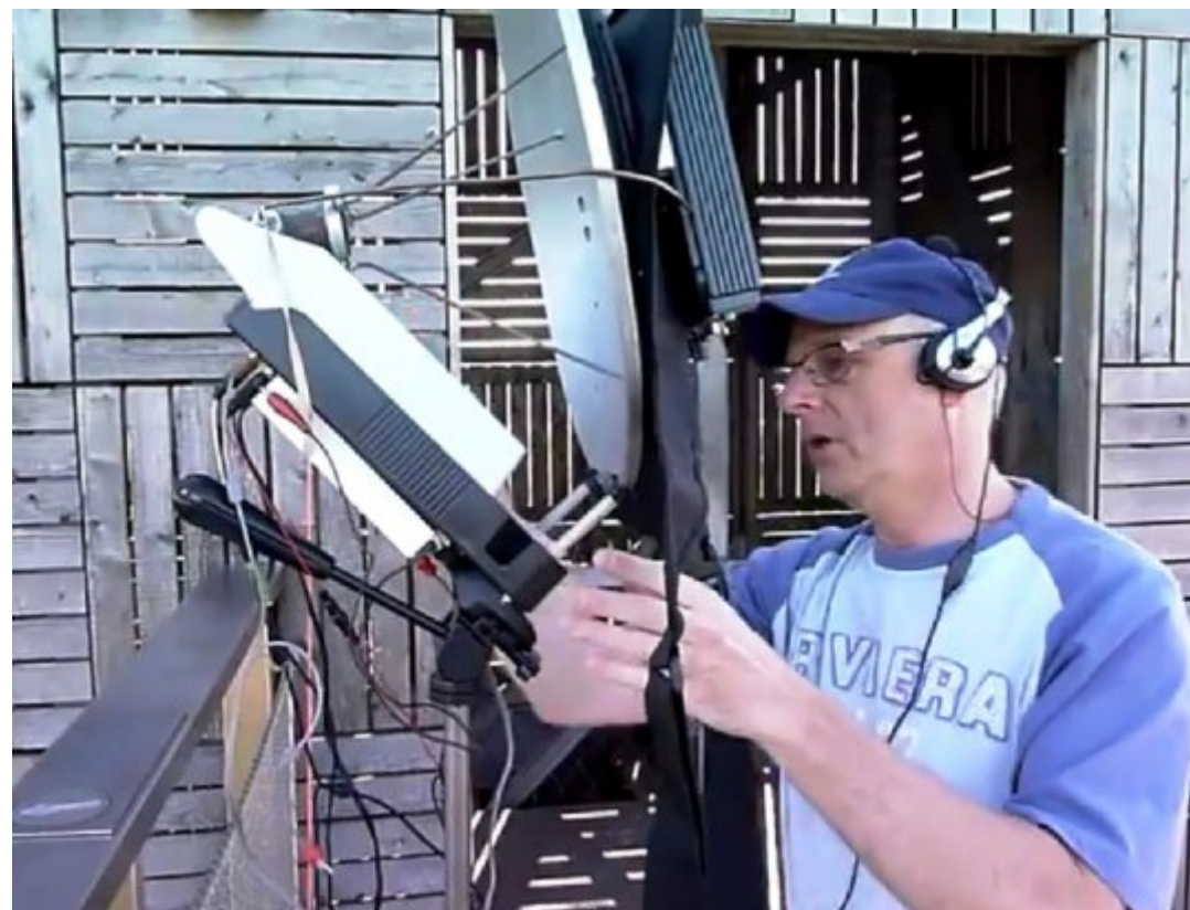
Prime focus dish from 6 cm station used as offset dish for 24 GHz by PA3CRX
