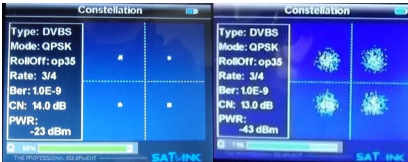
Fig 05 - On the left is the clean QPSK modulation Constellation from new second board etch layout. On the right is the noisy QPSK Constellation from the original board etch layout.
