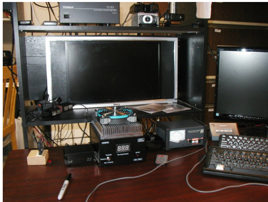
Left to right on upper shelf PA 12 volt supply 2 cameras [right is the 920] - left to right on desk cooling fan on block of wood, transmitter, box with power amp/12 V metering/antenna relay, receiver/small remote, power metering, etc
