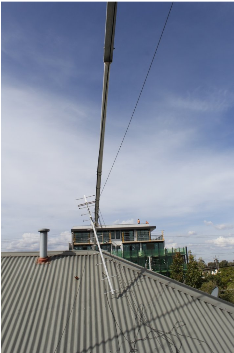
Mast lowered over next doors roof, 70cm ATV RX beam sighted to VK3RTV
