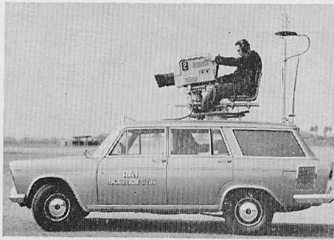
Fig. 1. Auto-top camera used in Italy.
