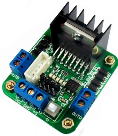
The motor drive amplifier module complete with L298 driver and associated components
