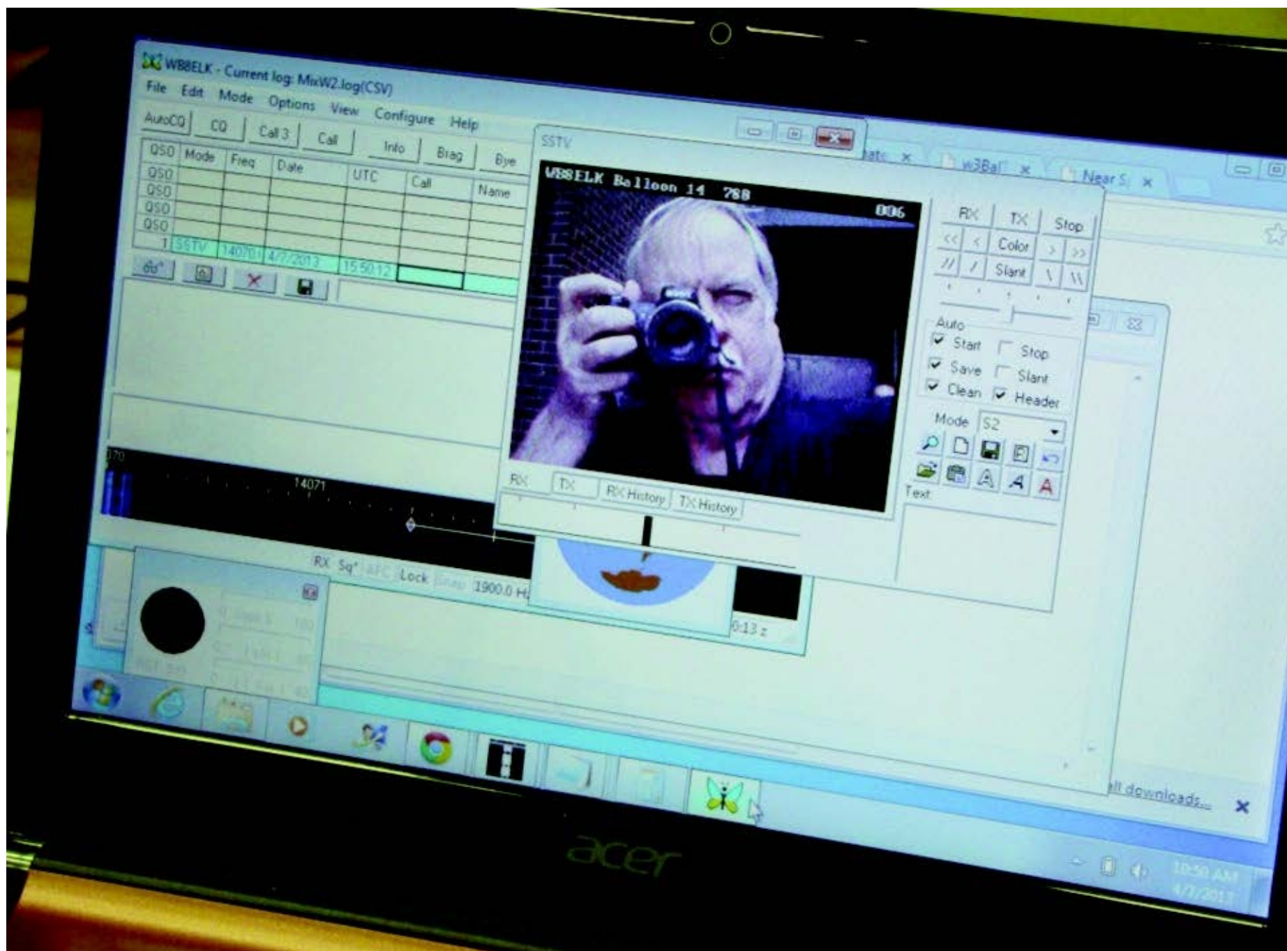
Using a netbook running MixW to decode the SSTV audio signal. Barry Lankford N4MSJ is captured taking a photo of the payload.
