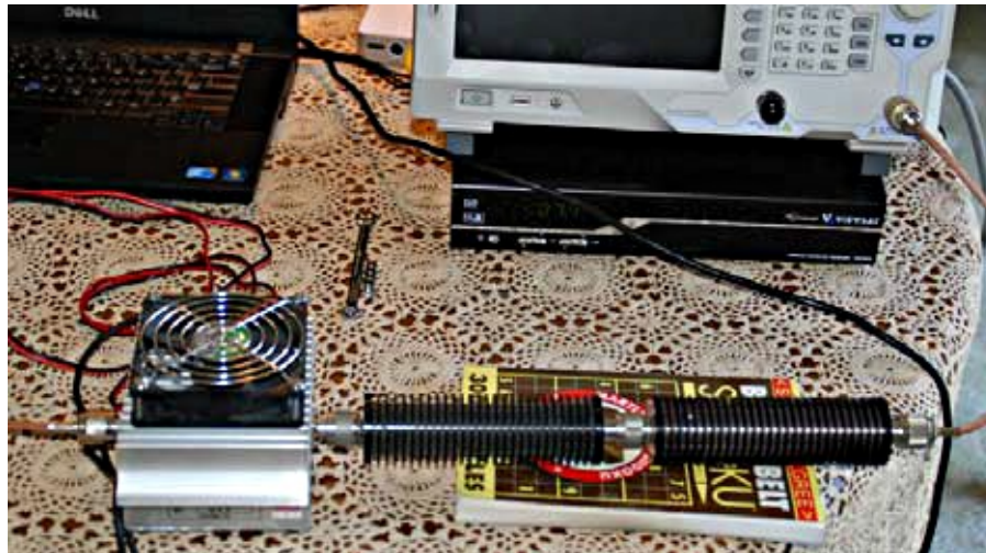
Figure 7 – The Down East RF Power Amp is connected to the Spectrum Analyzer through an
