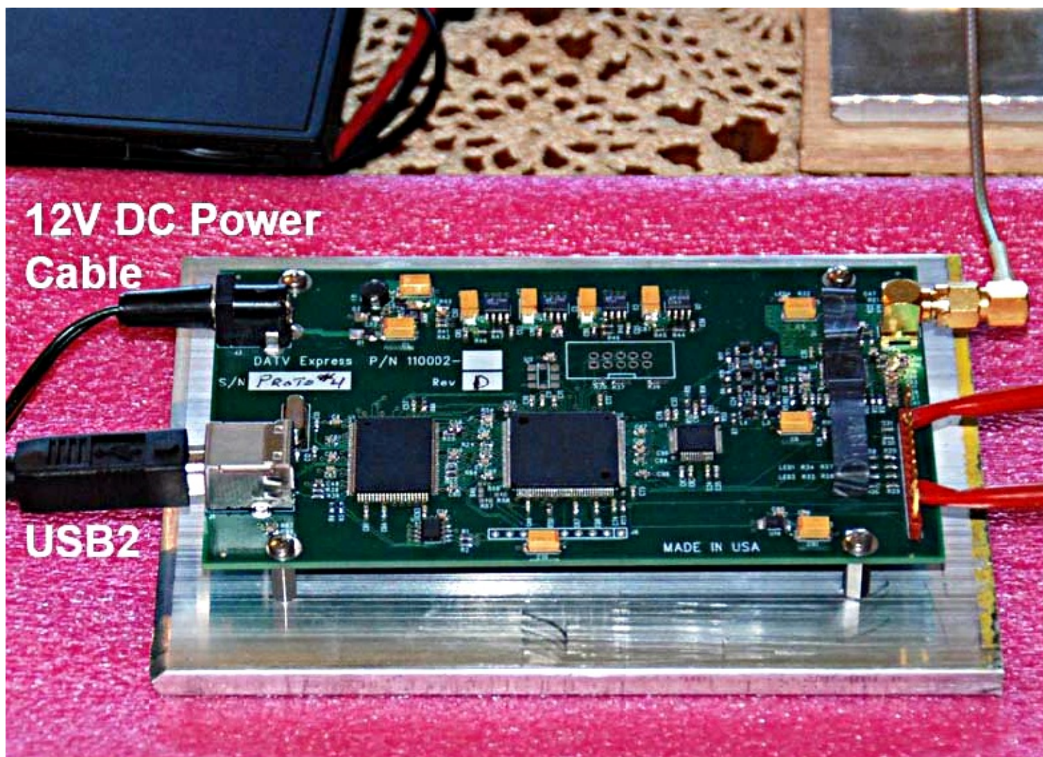
Figure 2 – The DATV-Express exciter hardware board is fitted with an aluminium plate as a heat-spreader
