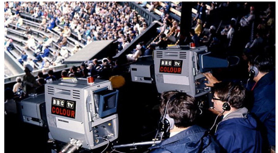
Philips PC60 Cameras, using 3 plumbicon tubes. Famous for using two camera cables
