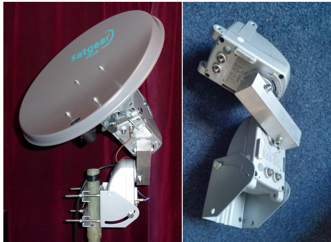
Left: 40cm dish for demonstration purposes Right: Positioners connected by a custom joiner bar. Photo and CNC milling: M0DTS
