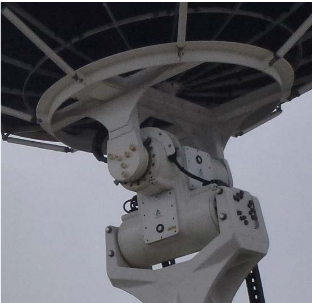
3.8m Catapult dish at Goonhilly used for tracking the ISS. Photo: G8GTZ
