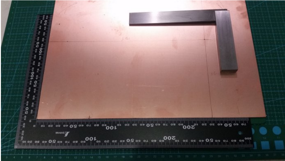
Double sided PCB – antenna reflector marked out 231 x 116 mm
