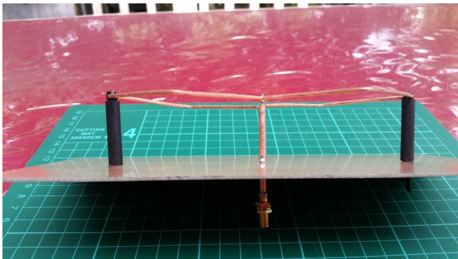
View of the driven element and coax feed line. Driven element ends are supported by plastic stand-off insulators
