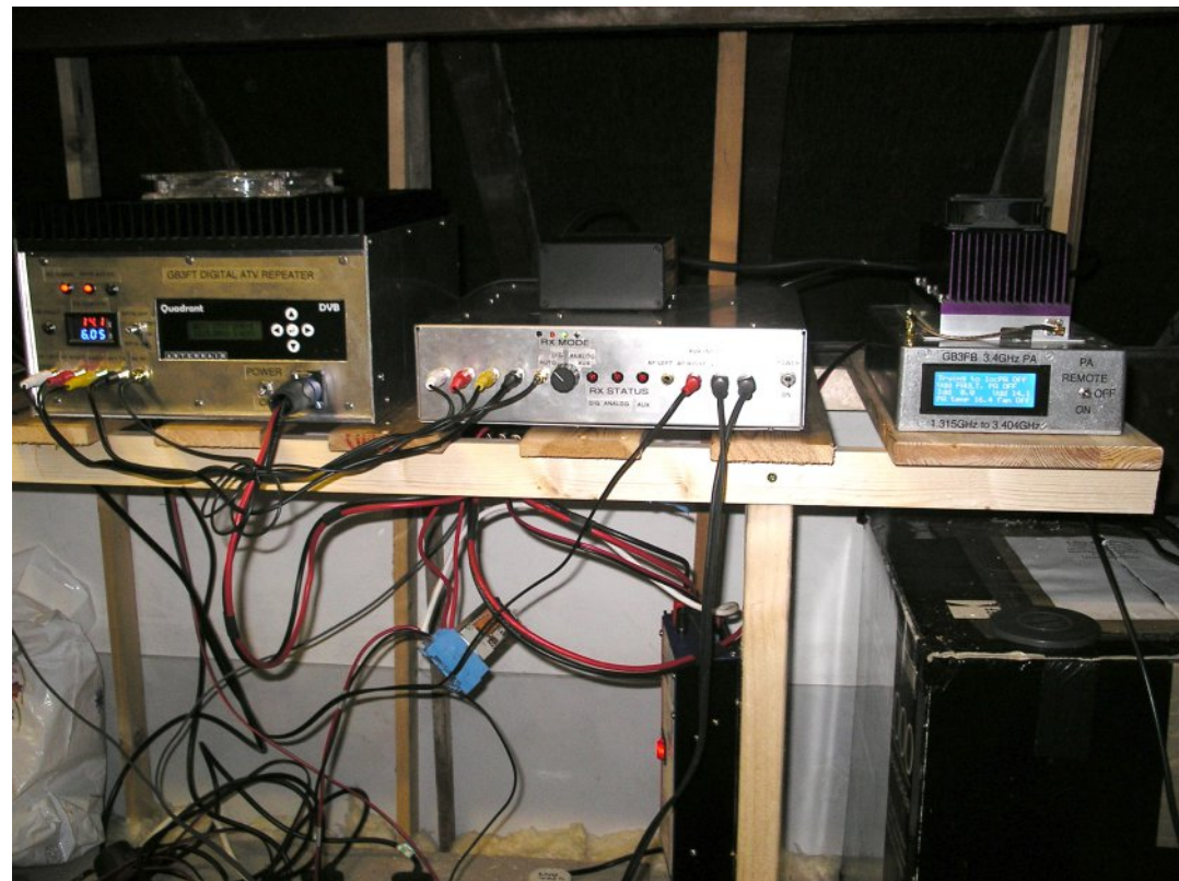
The 13GHz tx, the rx module and 3.4GHz PA all located in the loft space of G3WGU the repeater keeper
