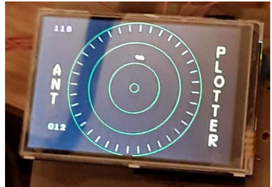
The TFT screen the display rings are set at 160 110 60, 10. 160 is the outer ring
