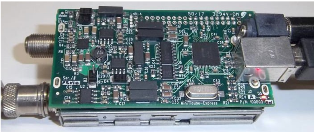
Figure 1 – Hand-soldered prototype using MiniTiouner-Express PCB with Serit NIM. The NIM lies flat underneath the PCB assembly.
