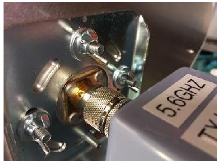
Above: Connecting the TX unit to the antenna Below: N type to RP SMA connector
