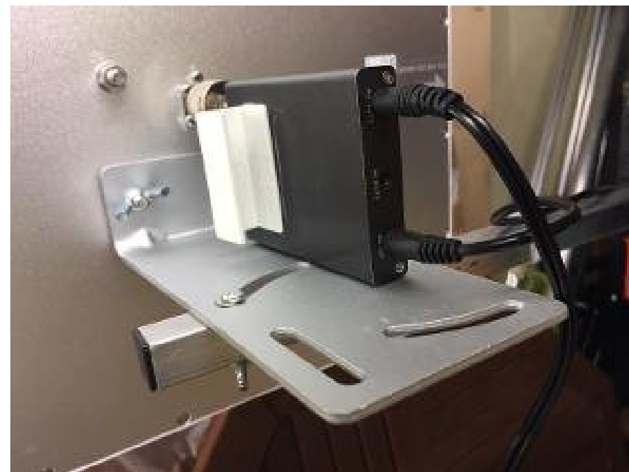
Fitting the antenna bracket to the boom for horizontal polarisation
