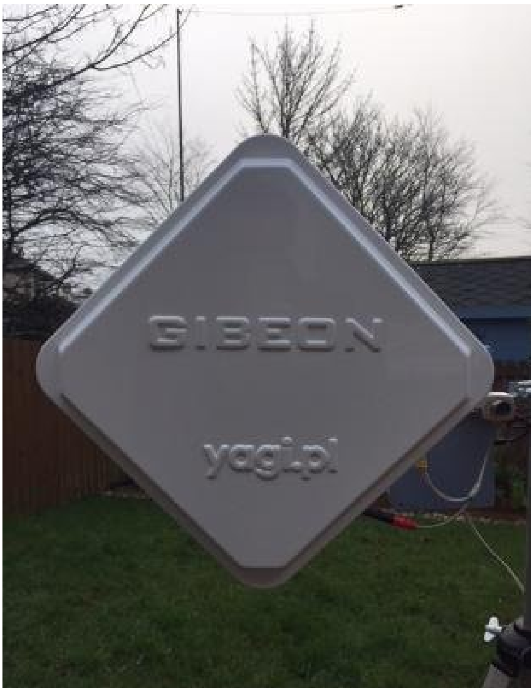
5Ghz 24dBi HV WIFI RP-SMA Wireless Signal Booster antenna by 'Gibeon'
