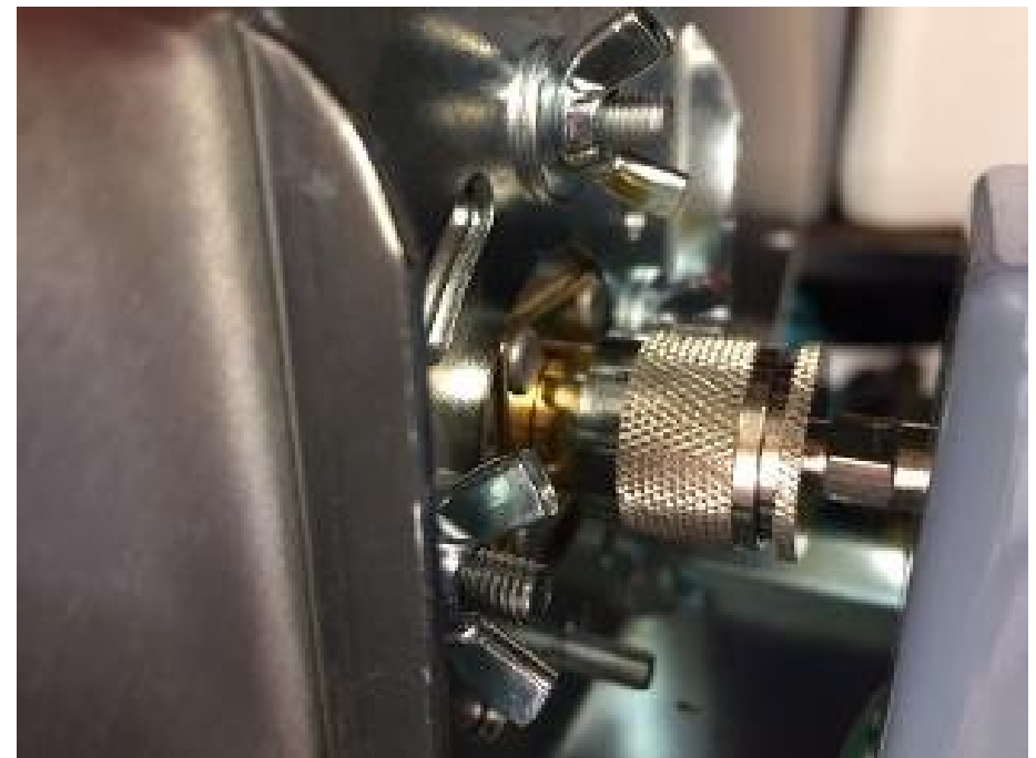
Above: Connecting the TX unit to the antenna Below: N type to RP SMA connector
