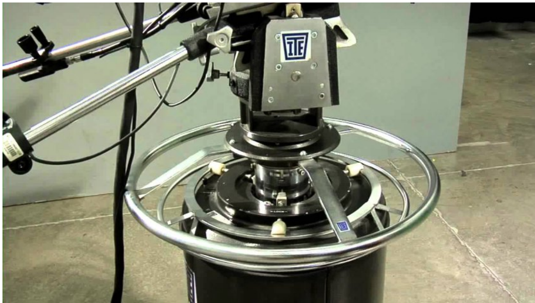
Typical stock shot of a Camera Pedestal, steering gear and the lower section where the lead weights go
