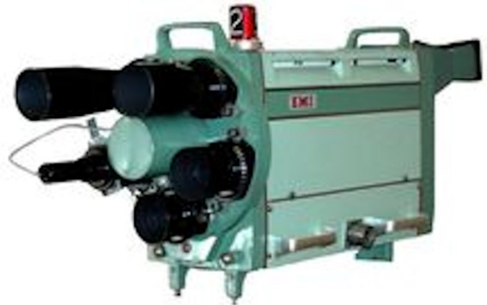
Camera head of an EMI 203 5 lens camera
