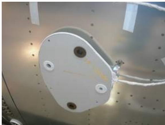
One of the Columbus Module 2.4 / 1.2 GHz Antennas
