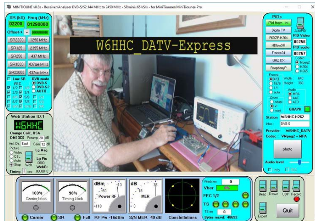
Screen-capture of v1.25LP7 software driving a DATV-Express board with DVB-S protocol. The audio was perfect.
