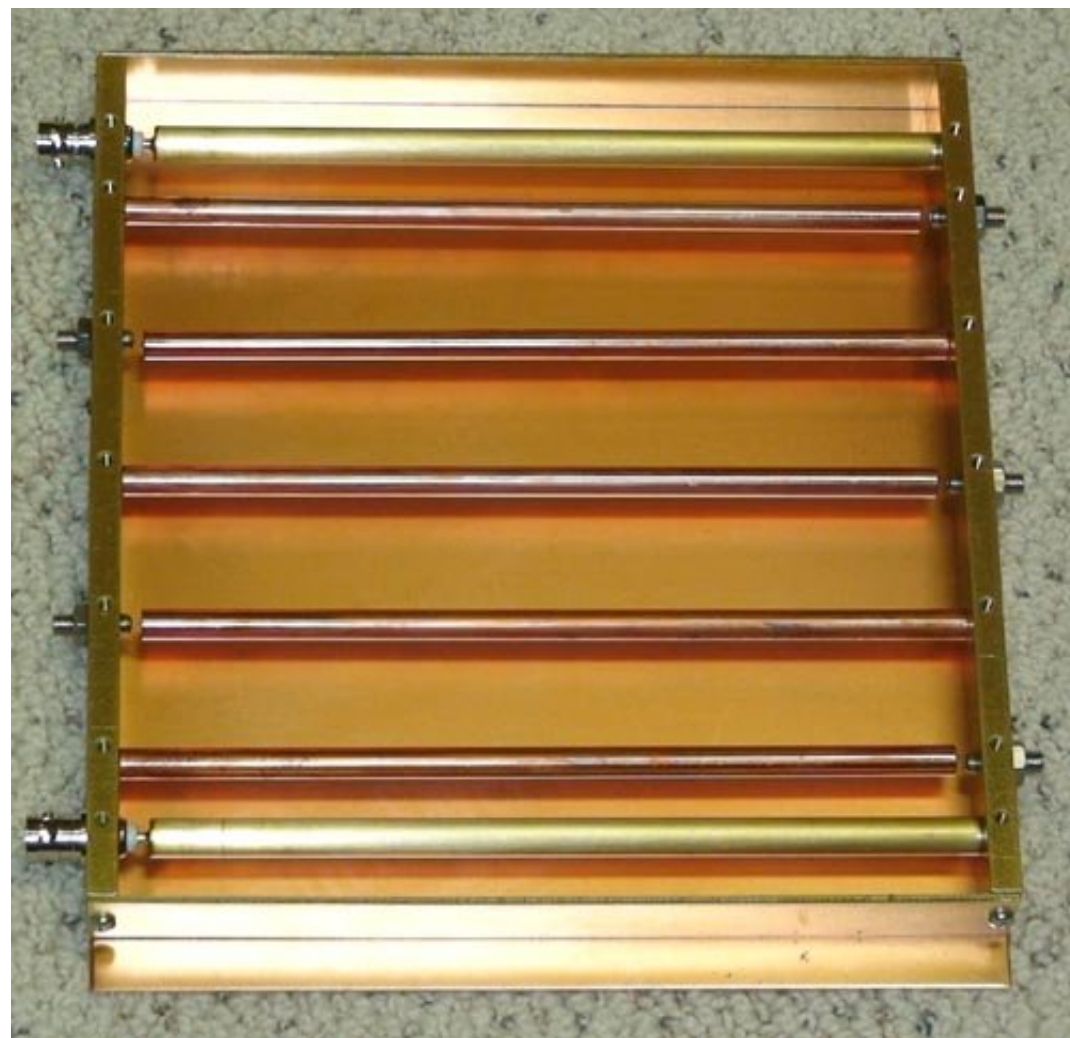
Fig. 2 Typical, 70cm, Inter-Digital Band-Pass Filter. Shown with top cover removed
