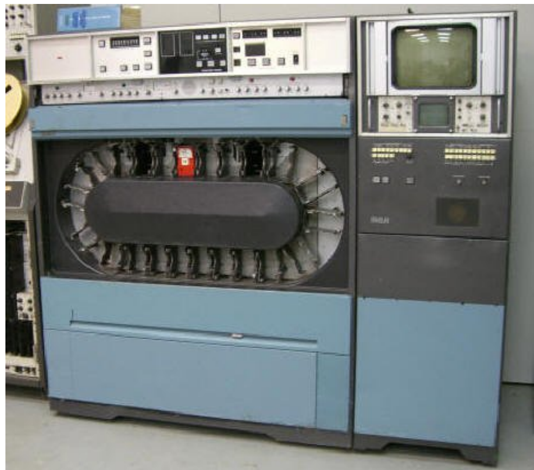
RCA TCR100 The distinctive Tank track rotates back and forth to deliver the correct cartridge to the deck loading arms
