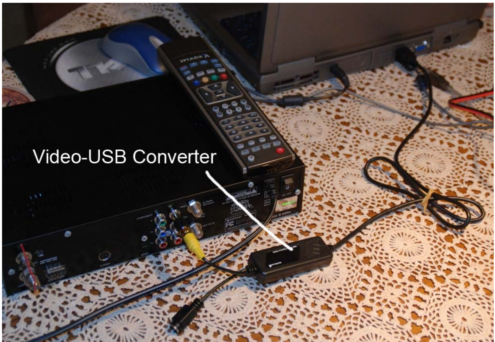
Figure 06 – The Startech video-capture unit converts STB video to USB
