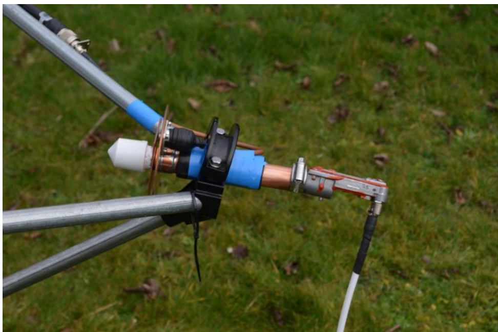
Above: Side-view of G4GUO Dual-Band-Feed for OSCAR-100 antenna
