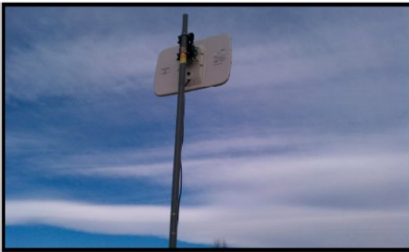
First year setup at the rest stop using a Ubiquiti PowerStation on a short mast and an analog NTSC camera that was converted to IP
