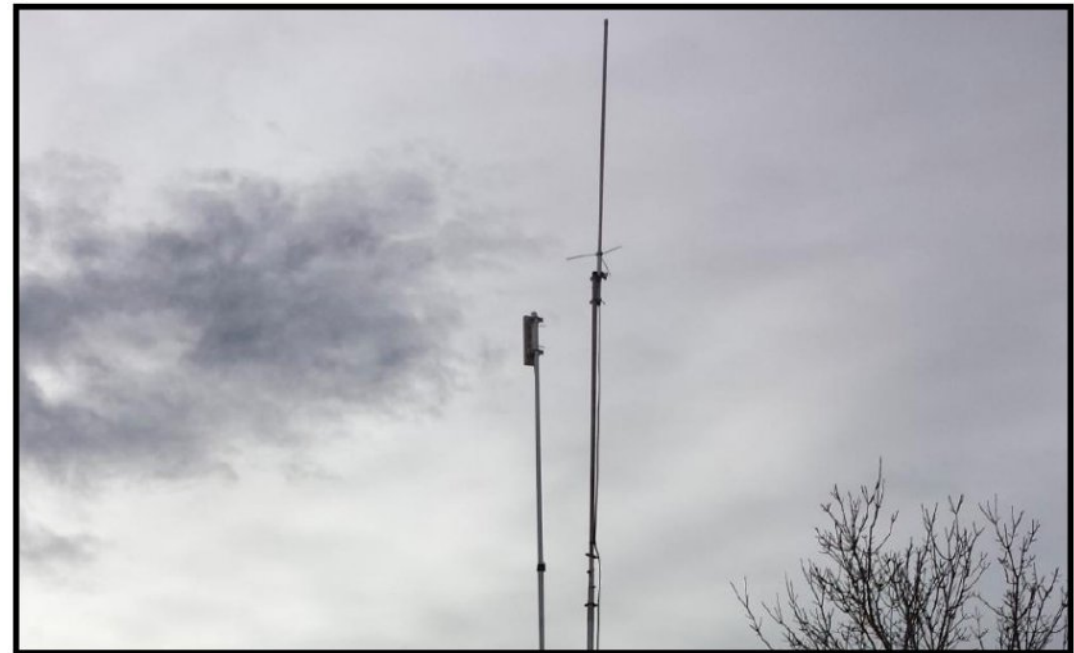
At the CP, a Ubiquiti 5 GHz. NanoStation on a push-up mast to the left of the dual band V/UHF vertical antenna
