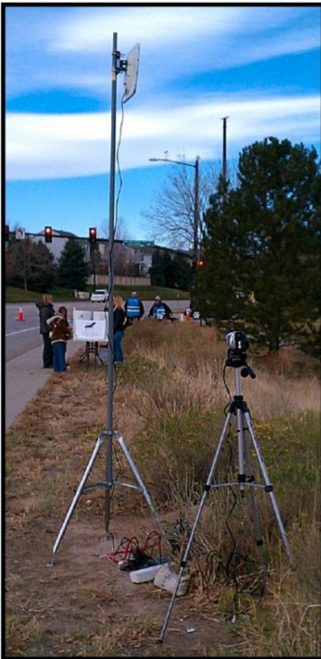
First year setup at the rest stop using a Ubiquiti PowerStation on a short mast and an analog NTSC camera that was converted to IP
