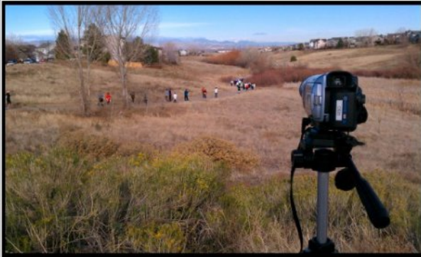
First year setup at the rest stop using a Ubiquiti PowerStation on a short mast and an analog NTSC camera that was converted to IP
