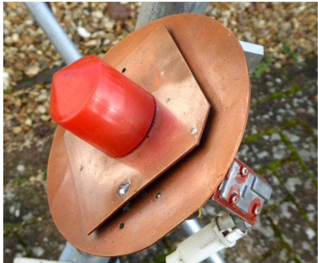
Figure 10 – Rocket LNB lens on patch
