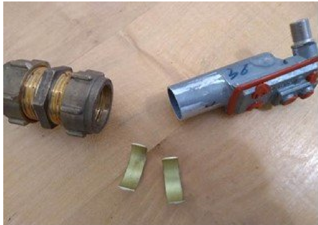
Figure 5 – Compression fitting for a decapitated LNB
