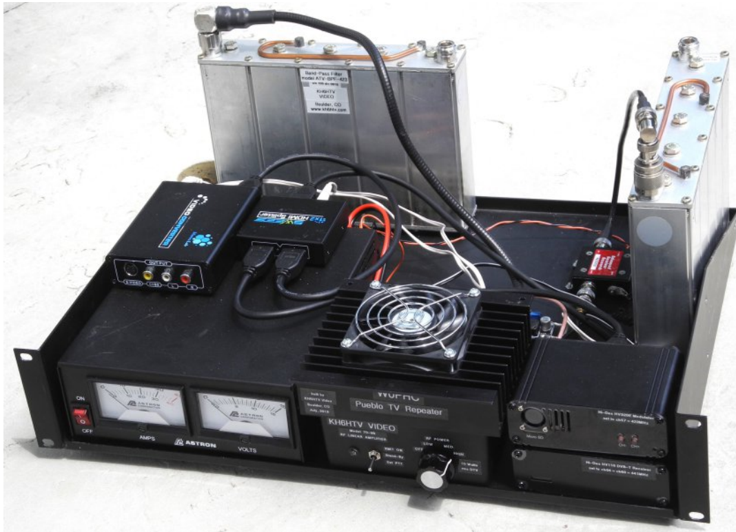
Fig. 1 A basic, 70cm, 10 Watt, DVB-T, Television Repeater
