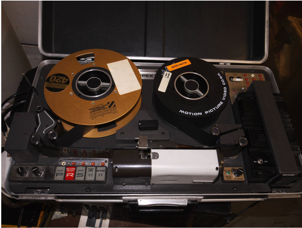
This is the actual machine made by Ampex to record Quadruplex in the field VR3000
