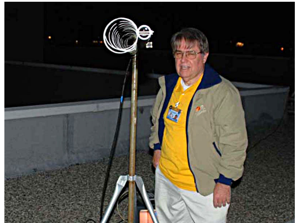
Figure 7 – Robbie KB6CJZ set up a 24-ele Loop-Yagi on the OPD roof and received perfect DATV pictures
