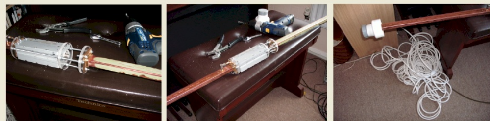
RX ANT to LNB then coax down to the RX in the Control Logic Box at the bottom of the mast
