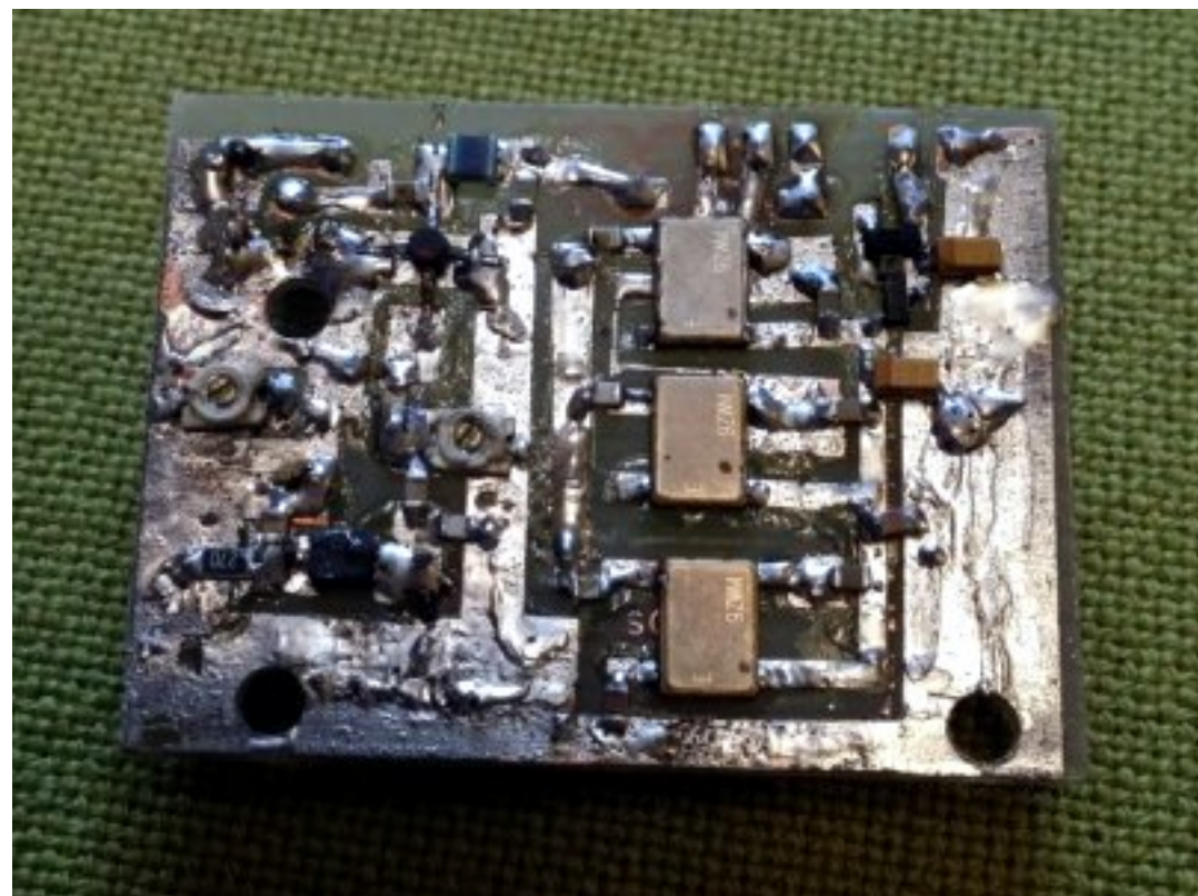
Foil & component side with the 3 Epson chips
