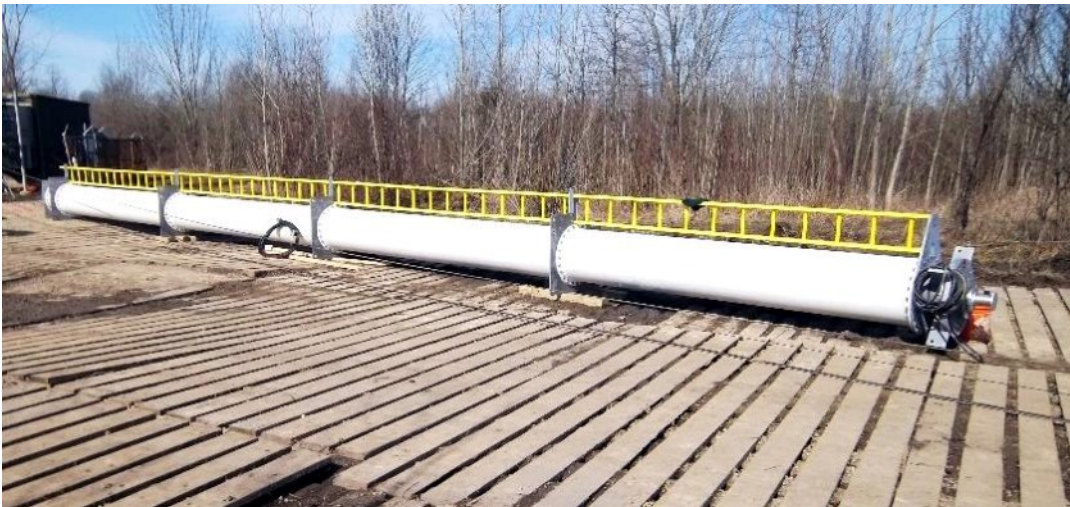
The new 55-foot-long multiple slot antenna. It's 32" in diameter and weighs 8800 pounds. Check out the ladder improvement over the old antenna. It's a standard Werner fiberglass ladder bolted to the antenna intermediate steel flanges
