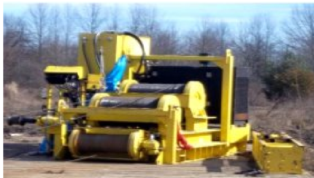
The winch used to hoist the antenna and workers up and down the tower. It holds 5000' of 3/4" cable
