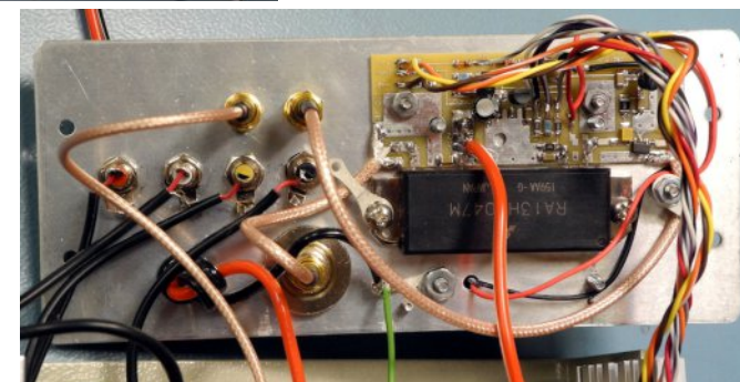
Rear panel with the 70-7, 10 Watt amplifier
