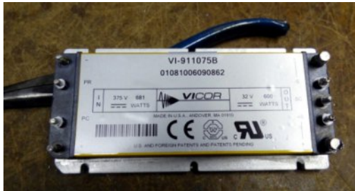
Power supply, 375VDC in, 32VDC out @ 18 A max.
