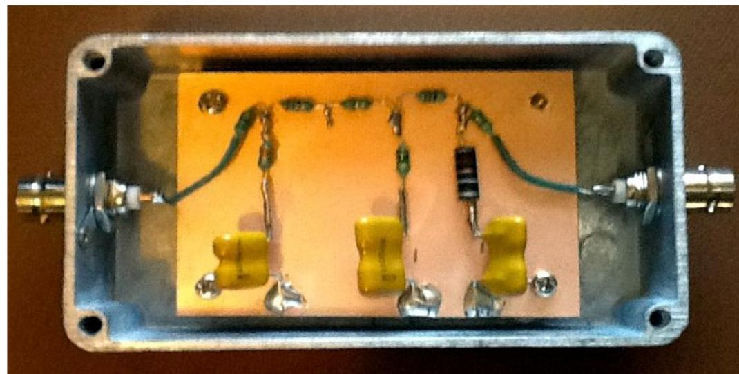
**Figure 1: The assembled 1 MHz lowpass video filter (housed in a Hammond 1590B enclosure)**
