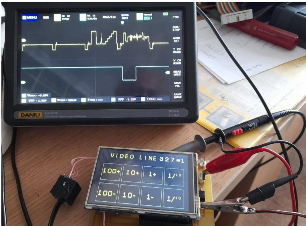
**Figure 2 - This was my scope trigger unit in action, and it shows video waveforms expanded in a way that the original unit was not capable of delivering as a stand-alone unit**
