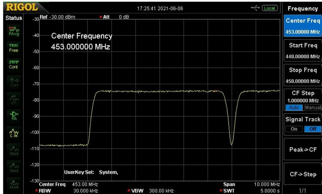
This (previous picture) shows the typical spectrum of a single TV channel. It is cable channel 62 (453MHz). 10dB/div & 1MHz/div. Resolution band-width was set to 30kHz. Note: there was no signal on Ch 61, but there is another signal present on Ch 63. Note the deep notch at the channel edge. The channel filter roll-off is thus preventing cross-talk into the adjacent channels. The noise floor of the measurement was about -109dBm
