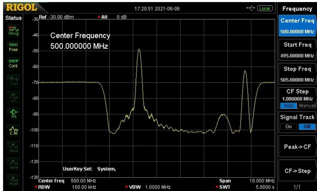
The exception was at 500MHz, where I found a single analog TV signal on channel 70
