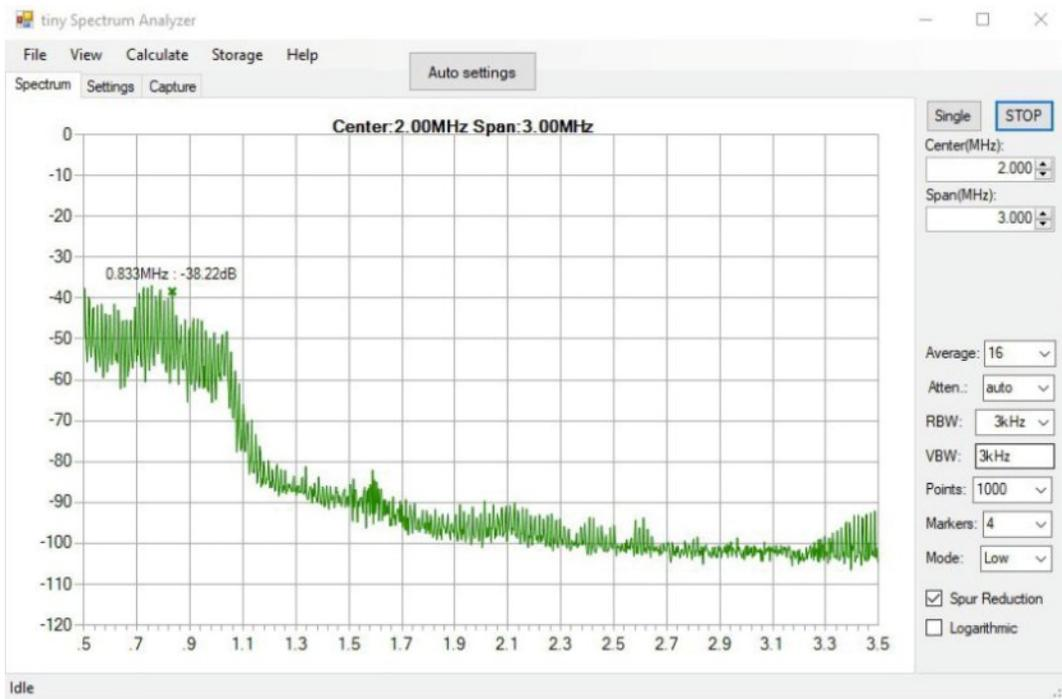
**Figure 2: The spectrum at the output of the 1 MHz low pass video filter, with its input fed from an NTSC video camera (measured with a tinySA® spectrum analyzer)**
