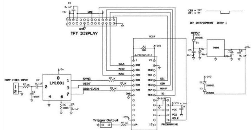
**Figure 3 - The scope trigger unit see the full article in CQ-DATV 95 in the download library**
