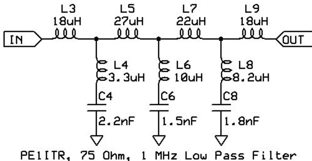
The author constructed the 1 MHz low pass video filter described by PA3CRX and PE1ITR. Above is the schematic diagram for the filter.
