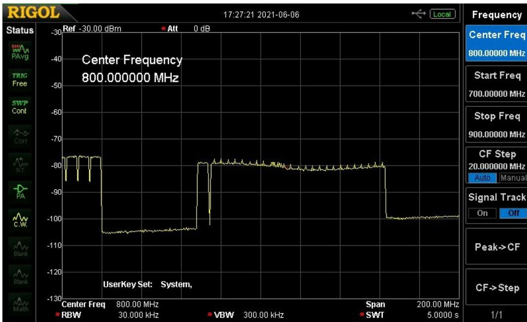
This is the region above 720MHz. Here we find one single DTV channel, but then a spectrum totally different from DVB-C. This appears to be a very wide, about 90MHz band-width digital signal with a bunch of pilot tones. This is for internet use. It is the "Down-Link" of data from the internet, plus whatever signaling the cable company needs to use.
