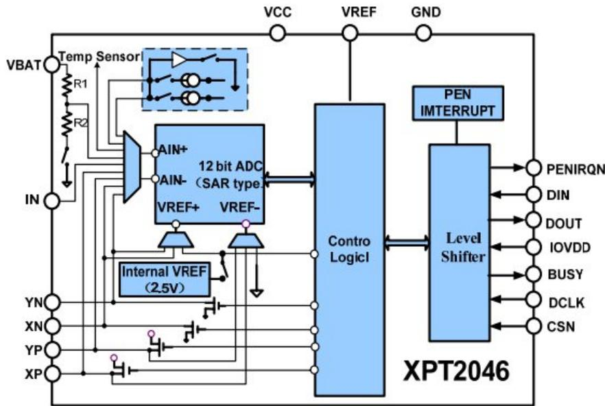
**Figure 4 - The basic operation of the XPT2046 is shown in this simplified diagram**
