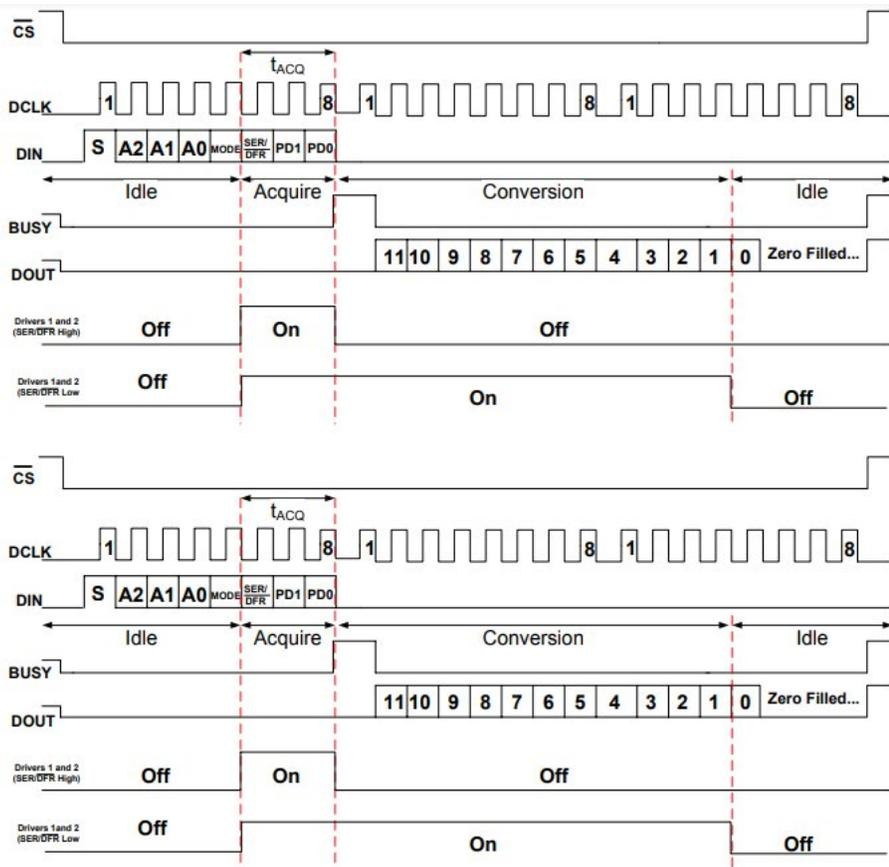
**Figure 6 - This is the protocol between the XPT 2046 and this PIC, as you can see there is lot happening**
