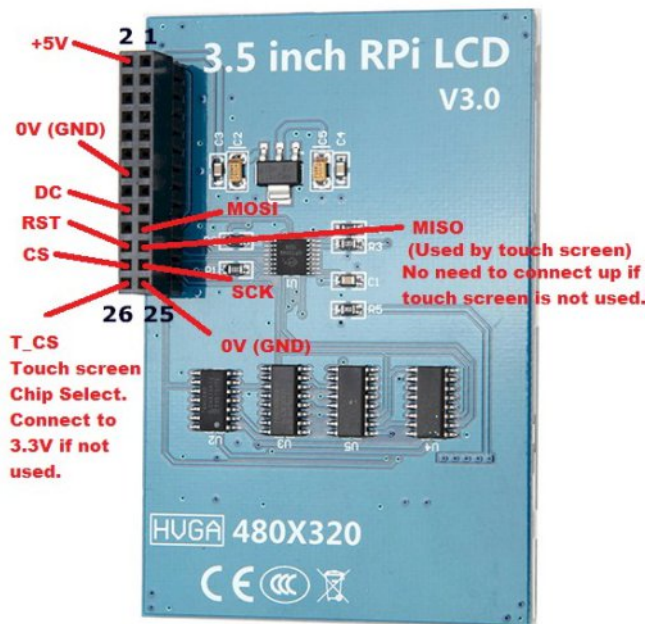
The touch screen driver uses SPI and is based on the XPT2046
