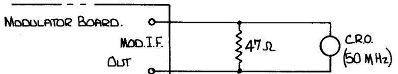
FIG.4 MODULATOR TEST
