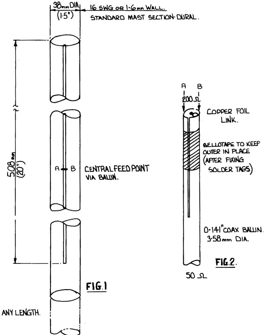
The length of tube beyond the slot is completely uncritical and the same tube could be used both as a mast and as an antenna! This includes the length of tubing above the short, so that either a simple short across the slot or a disc covering the top can be used, or the tube can be extended upwards in a similar manner to the bottom.
