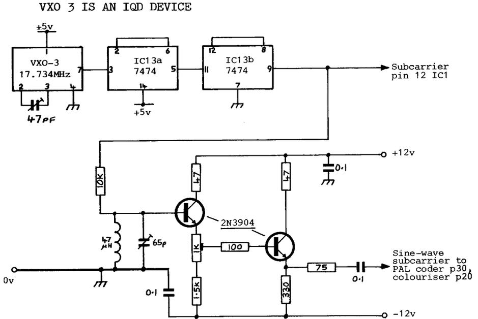
Fig.4 COLOUR SUBCARRIER OSCILLATOR (PAL)
